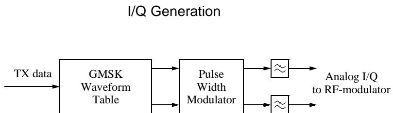
The RF signal characteristics follow the Mobitex Interface Specification, which defines GMSK with a  $B^*T$  of 0.3, +2 kHz deviation for a series of ones and -2 kHz deviation for a series of zeros.
