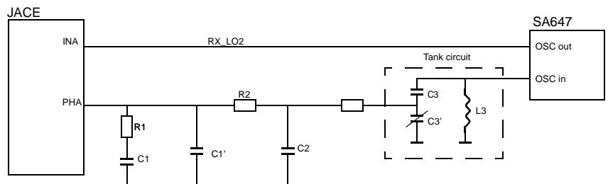
Loop filter and tank: R1, C1 and C1' sets loop performance, R2 and C2 attenuates the phase detector frequency and L3, C3 and C3' is the resonant tank circuit. C3' is a varactor diode, which is the tuning element in the tank.
