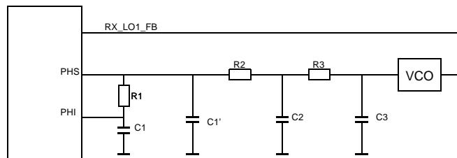
R1, C1 and C1' sets loop performance, R2 and C2 attenuates spurious caused by channel spacing fractional counters, and R3 and C3 attenuates the spurious at the phase detector frequency.
