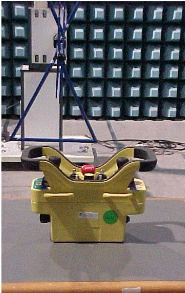
PHOTO N° 2 – SET-UP FOR EMISSION RADIATED TEST
