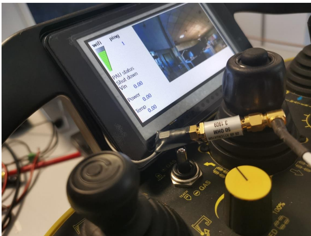
Figure D.5: further details of radio remote controller and the passband filter
