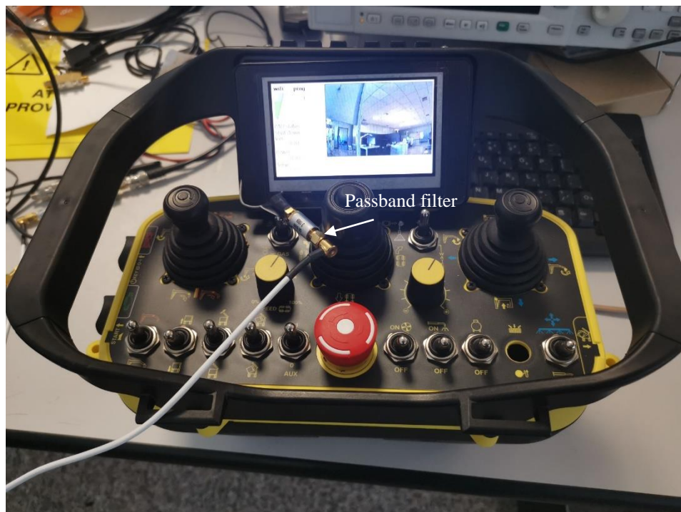
Figure D.3: Radio Remote Controller with Wi-Fi Sink with passband filter
