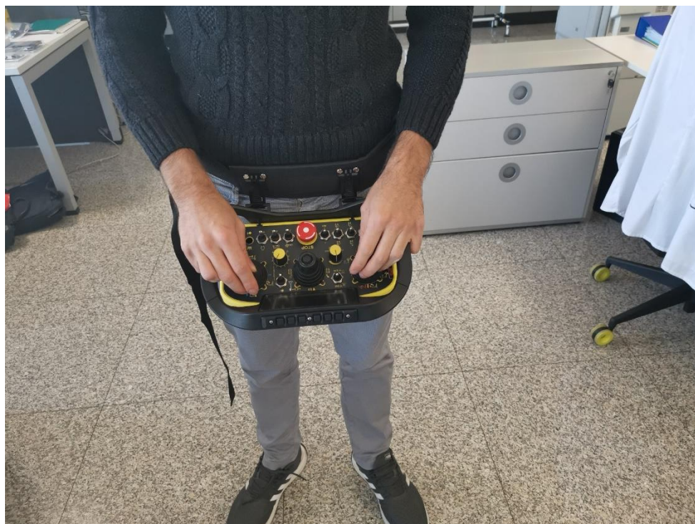
Figure F.13: Correct working position using PJM unit with belt and with hand on the unit, front view
