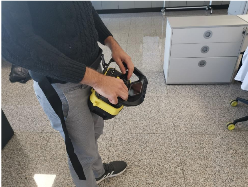
Figure F.12: Correct working position using PJM unit with belt and with hand on the unit, lateral view
