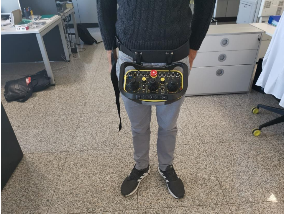
Figure F.10: Correct working position using PJM unit with belt, front view
