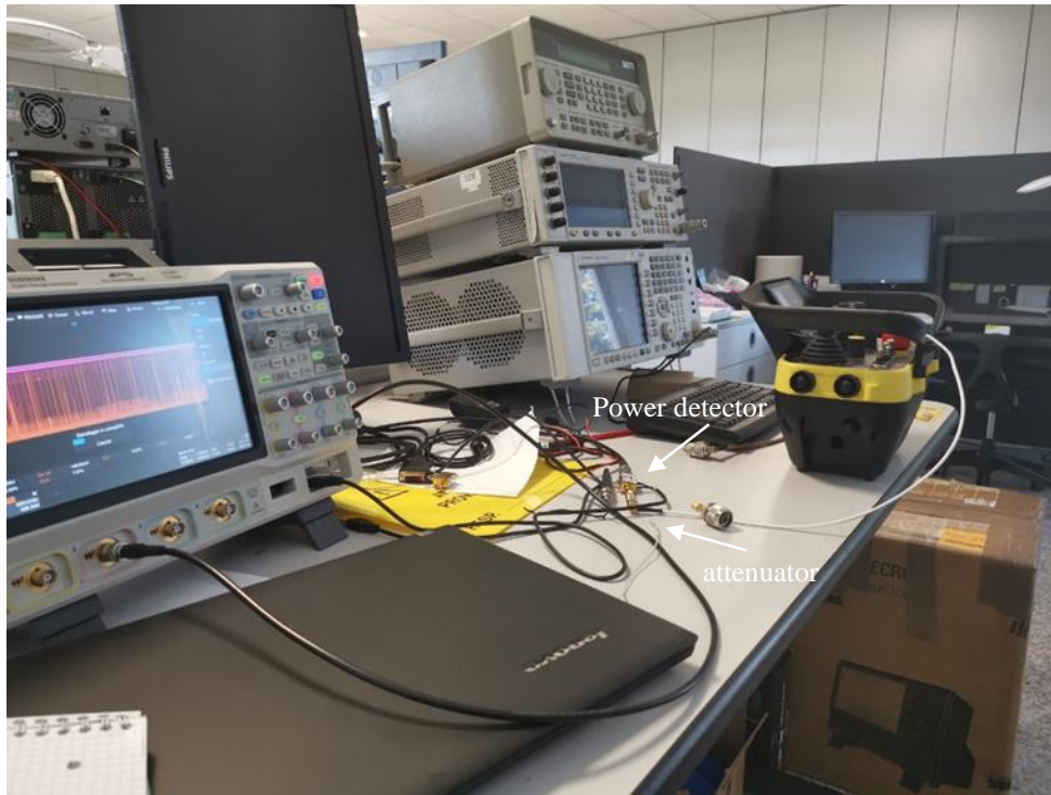
Figure D.4: oscilloscope, Radio Remote Controller with Wi-Fi Sink , attenuator and power detector
