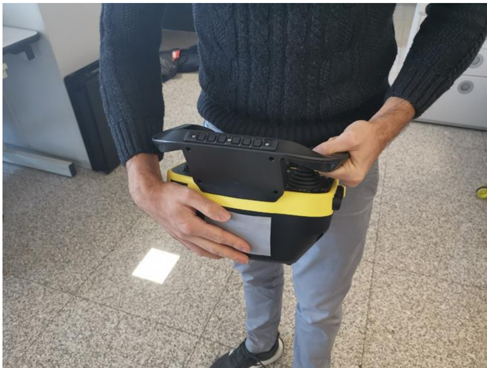
Figure F.8: Worst case working position for limb using PJM unit, front view
