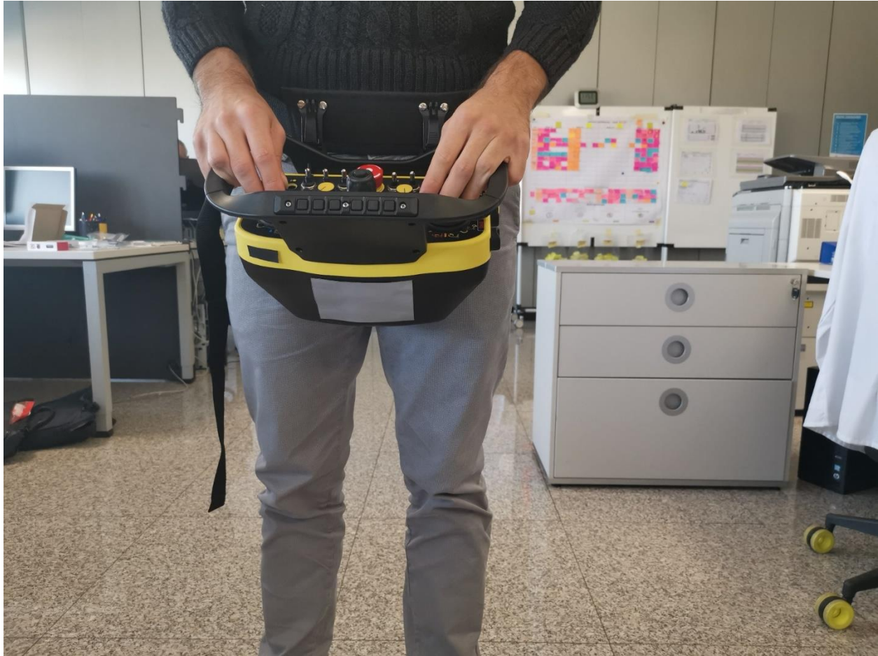
Figure F.14: Correct working position using PJM unit with belt and with hand on the unit (with additional details about the internal positions of antennas), front view
