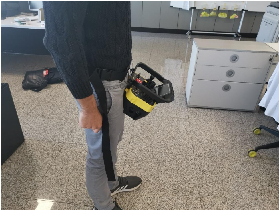
Figure F.11: Correct working position using PJM unit with belt, lateral view
