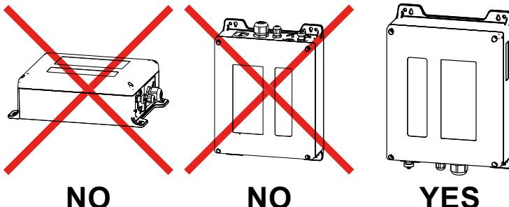
Fix the Base station in four points, using the specific holes in the housing.
