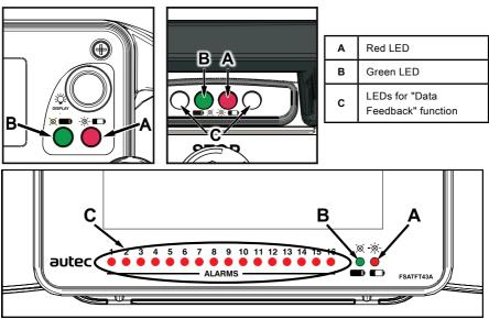
The DJM Transmitting Unit always has a green LED [B] and a red LED [A] that provide information regarding the Radio Remote Control.
