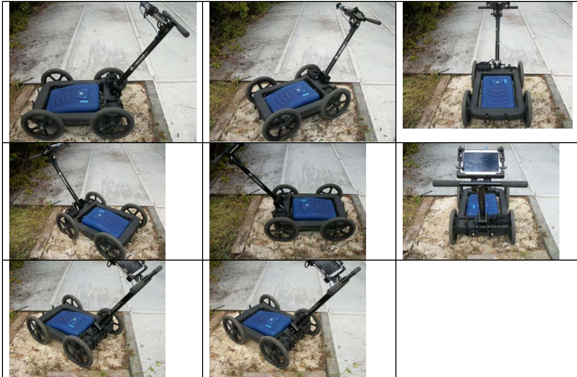
EUT Positions with 45 Degree Interval
