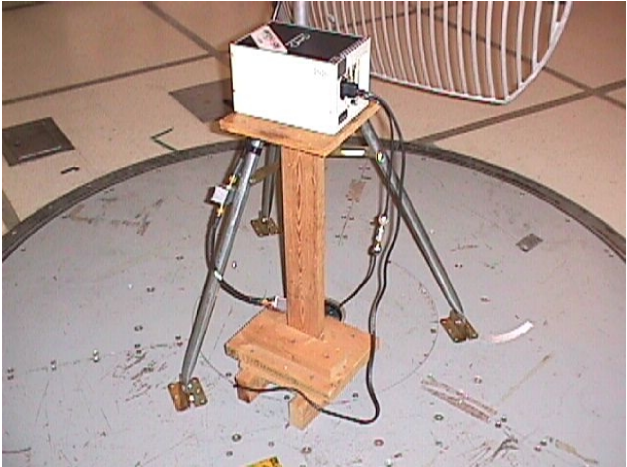
View of the Waverider NCL 1000 module during the Radiated Emissions tests.
