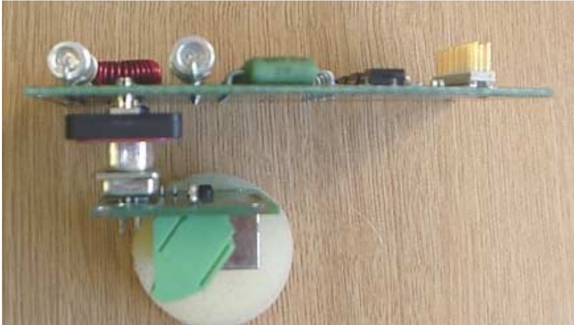
External Cable Interface and Lightning Protection Assembly
