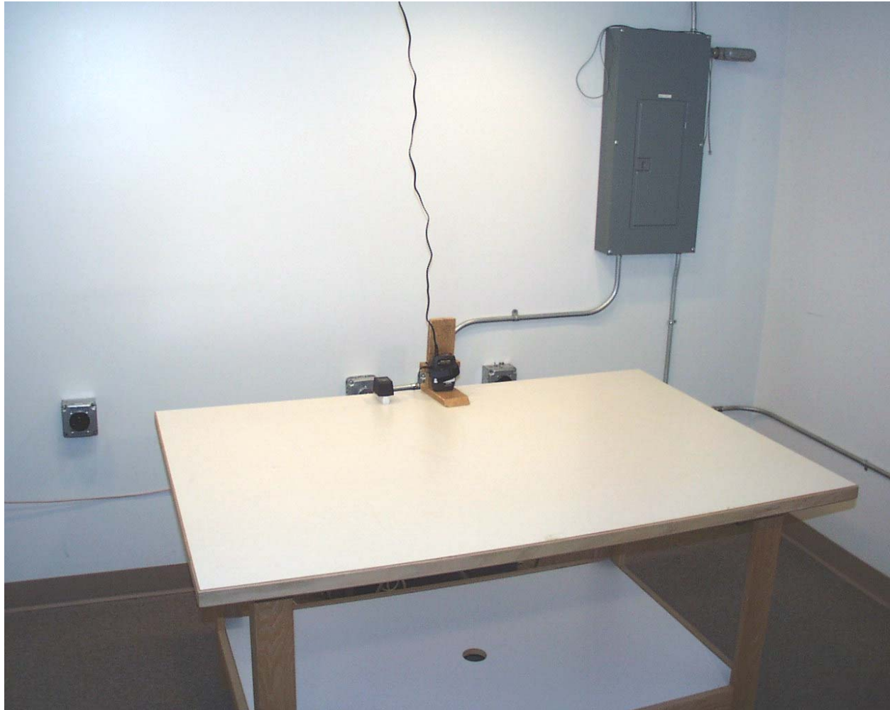
Photograph 5 - Front View Conducted Emission Setup
