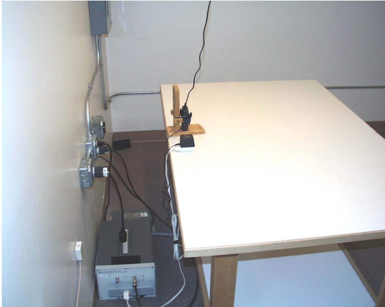
Photograph 6 - Rear View Conducted Emission Setup
