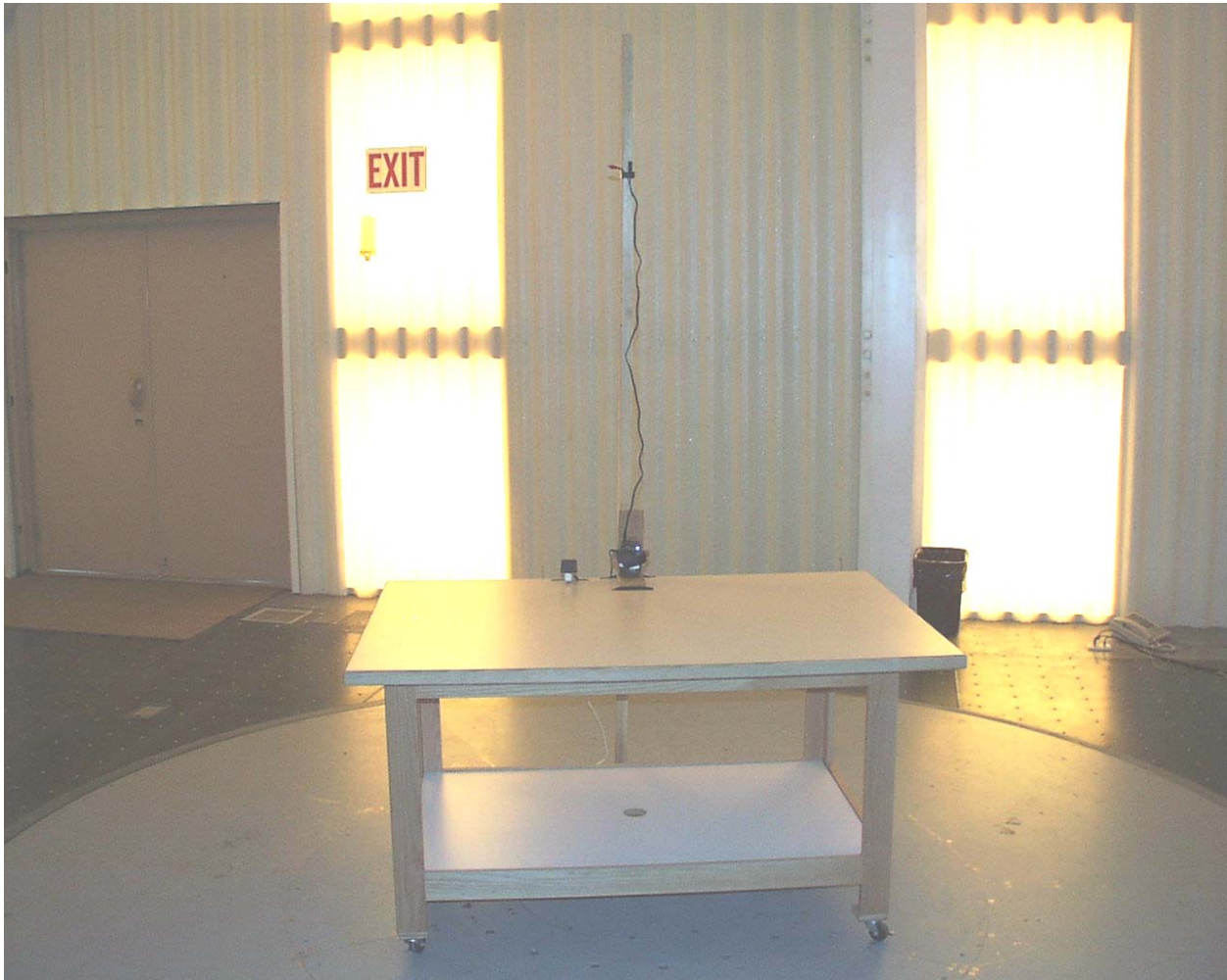
Photograph 1 - Front View Radiated Emission Configuration (Vertical Orientation)
