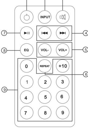
(1) Press this button to turn on/off the system power. This button will not turn on/off the AC power.
