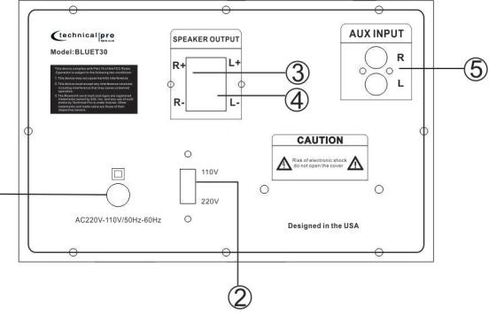
1. Power Supply: Connect the power cord here. The power switch (blue key on the front panel) should be set off position before the power supply is connected.
