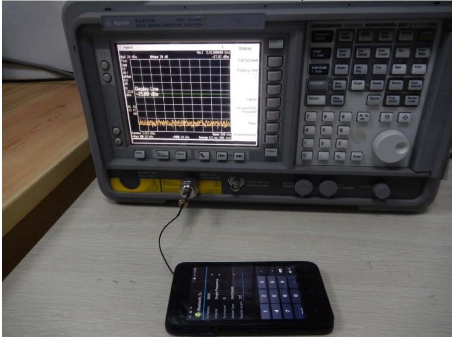
DSS&DTS RF conduction test photos
