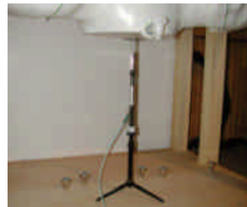
Figure 12.1 Dipole Validation Test Setup
