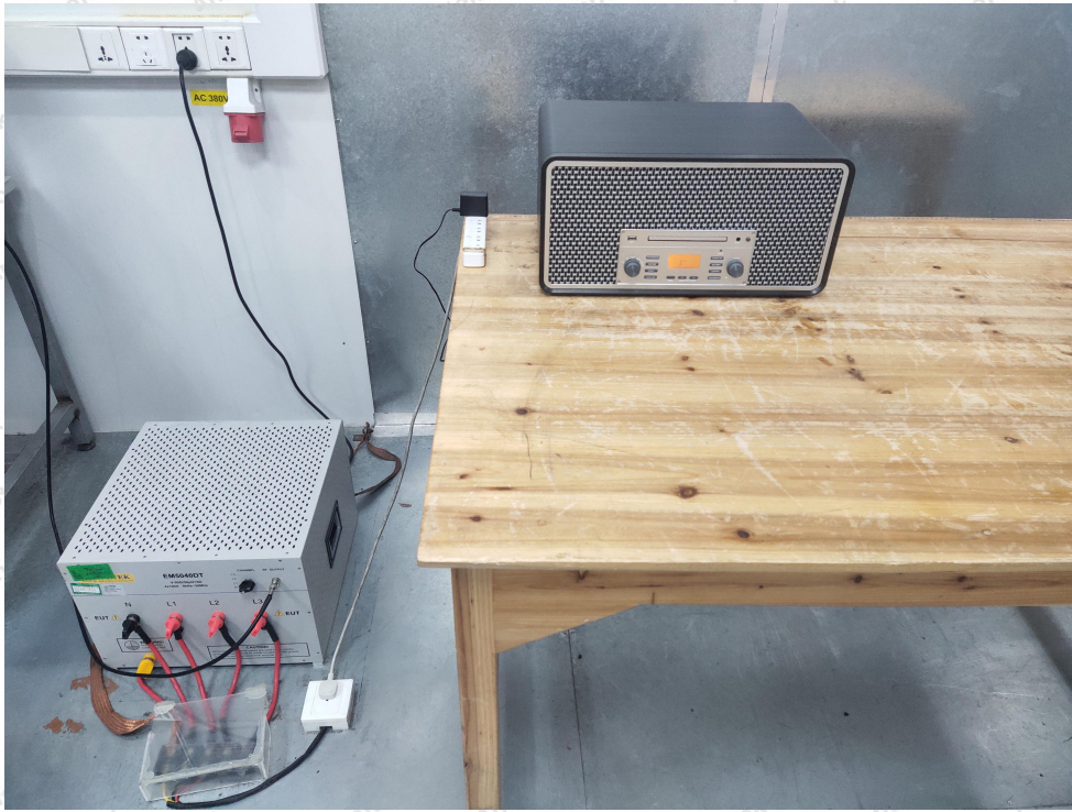
Photo of Conducted Emission Measurement
