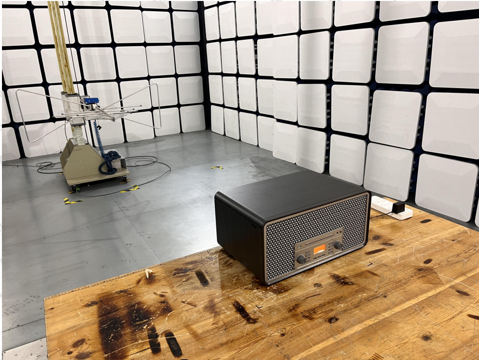
Photo of Radiation Emission Test
