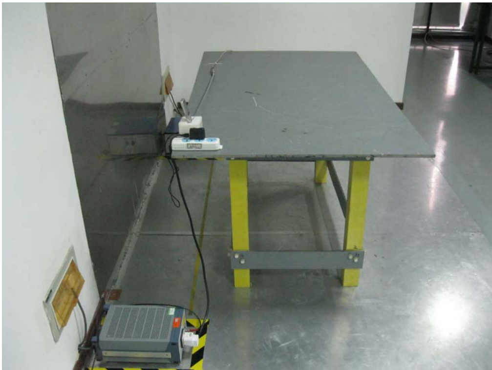
Conducted Emissions Test Setup - Side View
