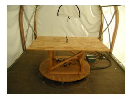
**Radiated Emission Setup - Rear View**
