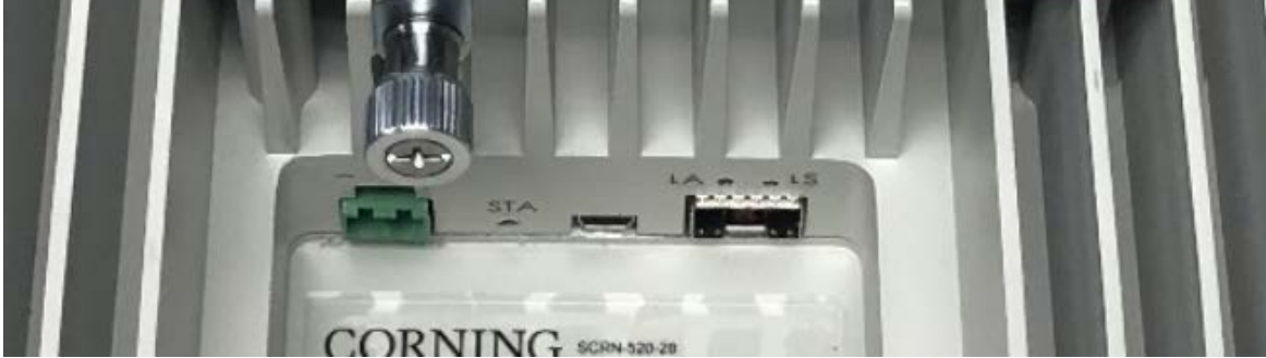
Figure 4 SCRN-530 Connectors and Status LED
