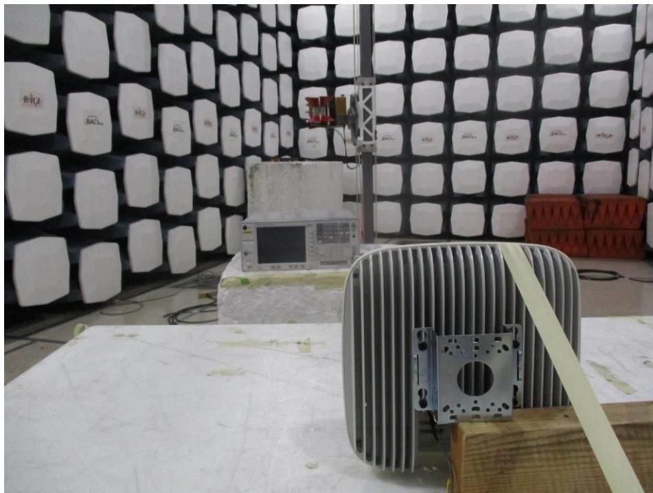
**1.10 Radiated Spurious Emission 40-100 GHz at 1 meter Rear View**
