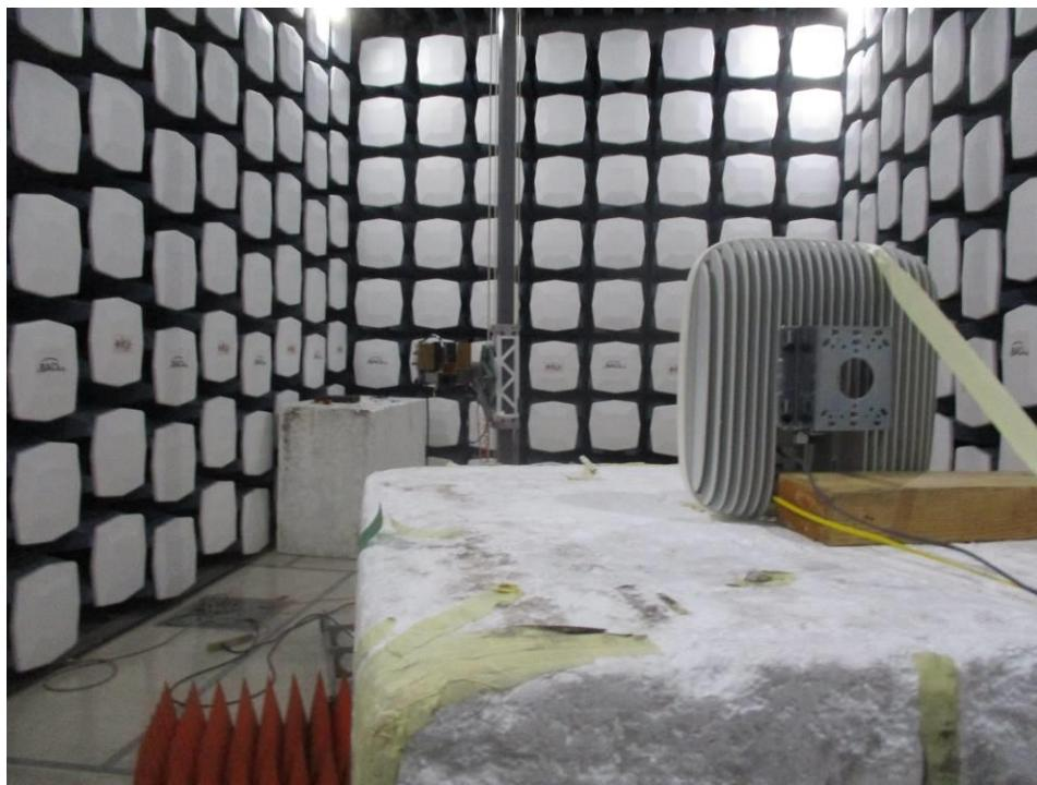
**1.9 Radiated Spurious Emission 40-100 GHz at 1 meter Front View**
