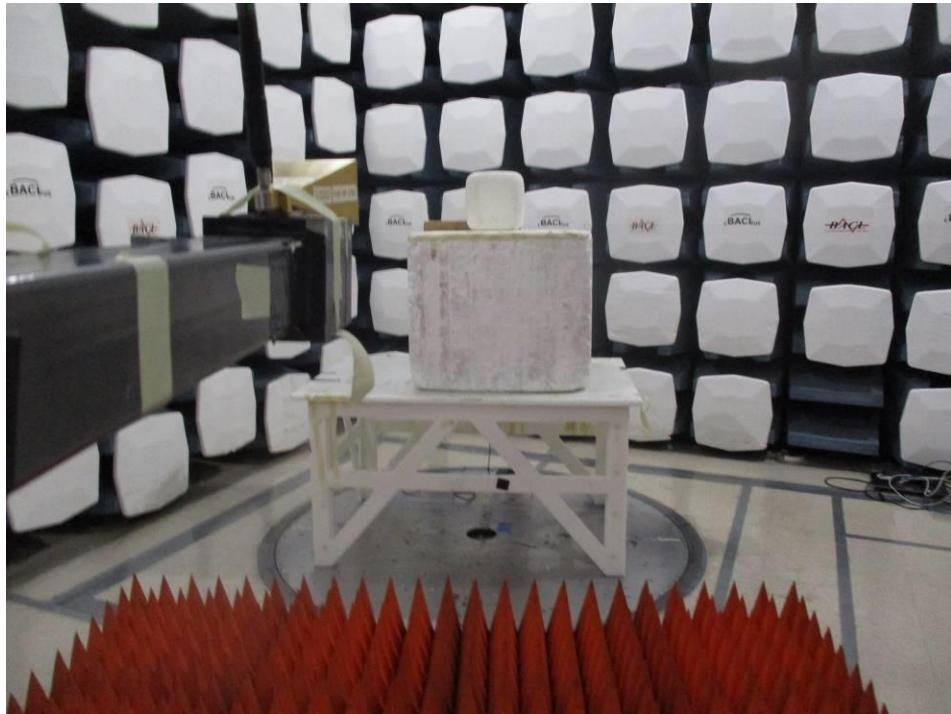
**1.8 Radiated Spurious Emission 26.5-40 GHz at 3 meters Rear View**
