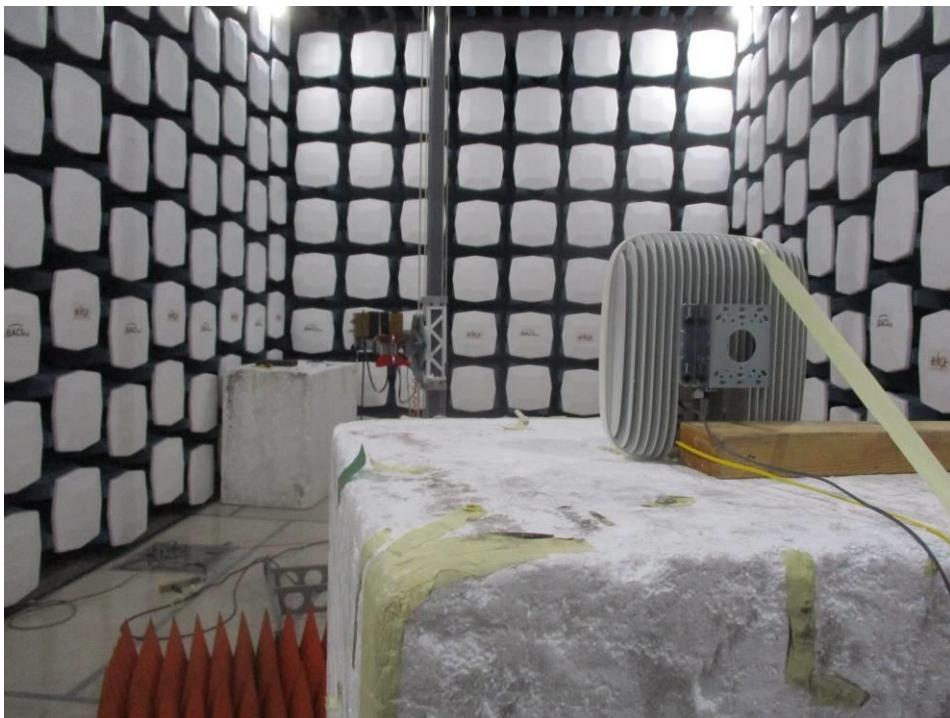
**1.5 Radiated Spurious Emission 18-26.5 GHz at 3 meters Front View**
