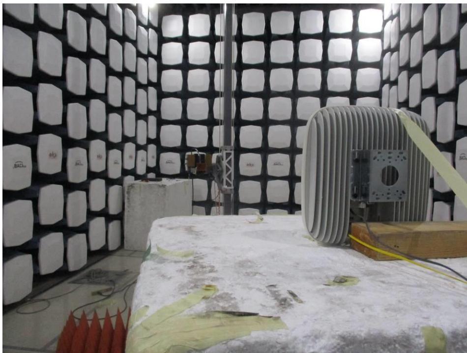
**1.7 Radiated Spurious Emission 26.5-40 GHz at 3 meters Front View**
