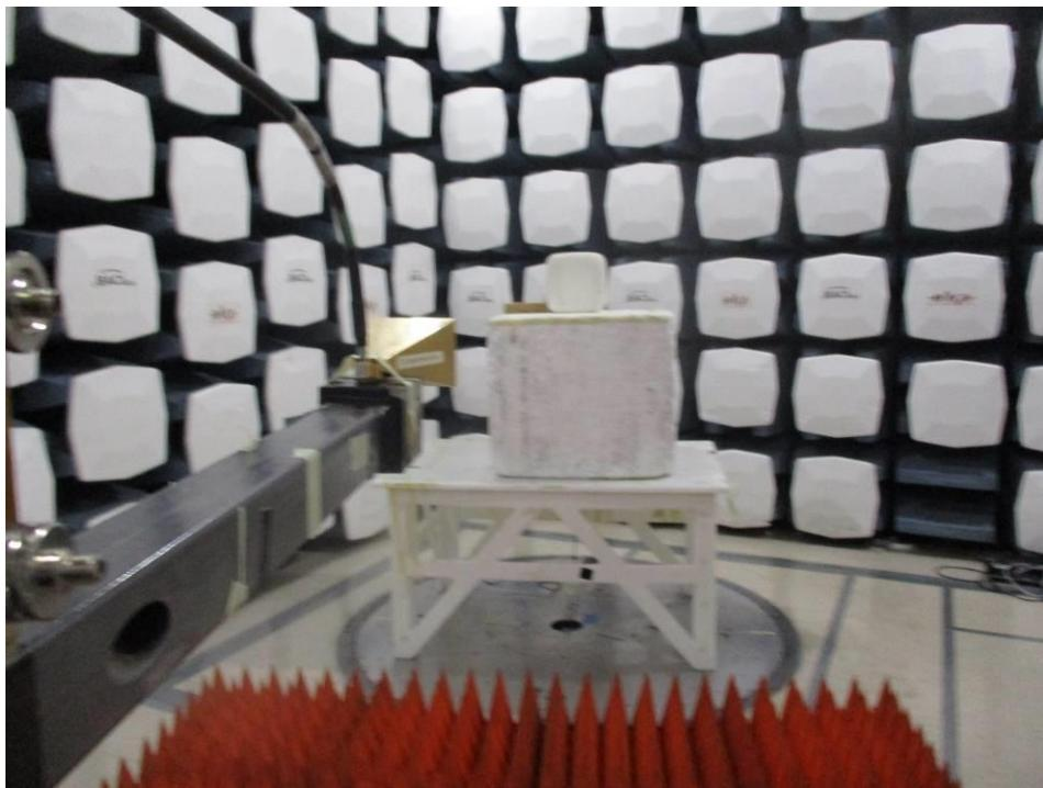
**1.6 Radiated Spurious Emission 18-26.5 GHz at 3 meters Rear View**
