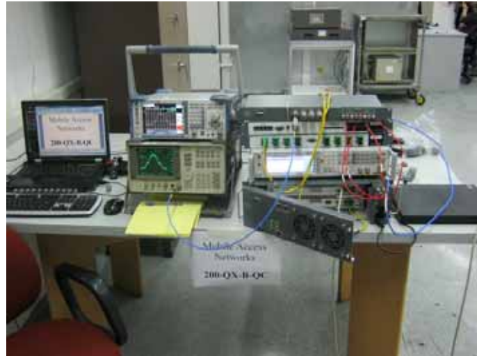
Figure 2. Conducted Emission From Antenna Ports Tests
