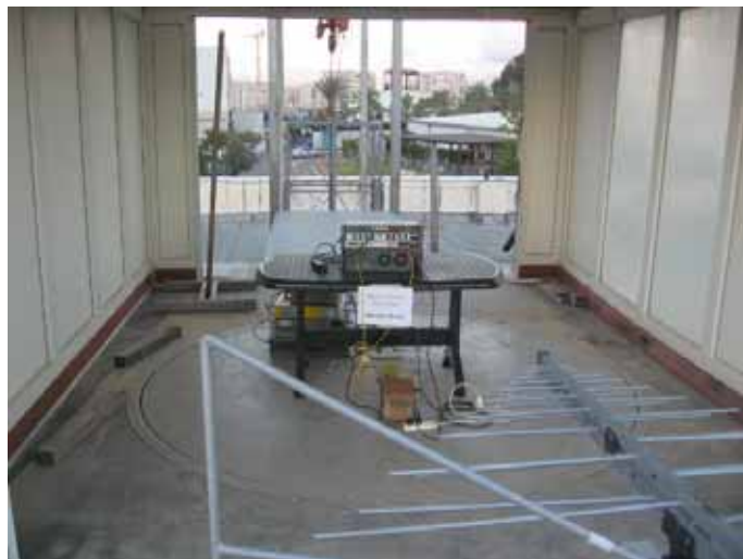
Figure 3. Radiated Emission Test
