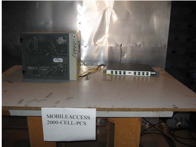
Figure 2. Conducted Emission From AC Mains Test Set-up
