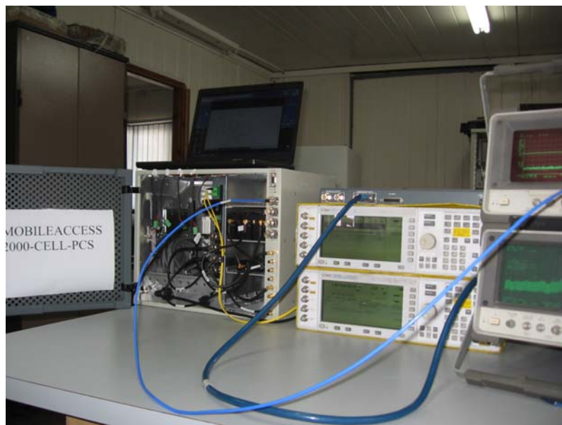
Figure 3. Conducted Emission From Antenna Port Test Set-up
