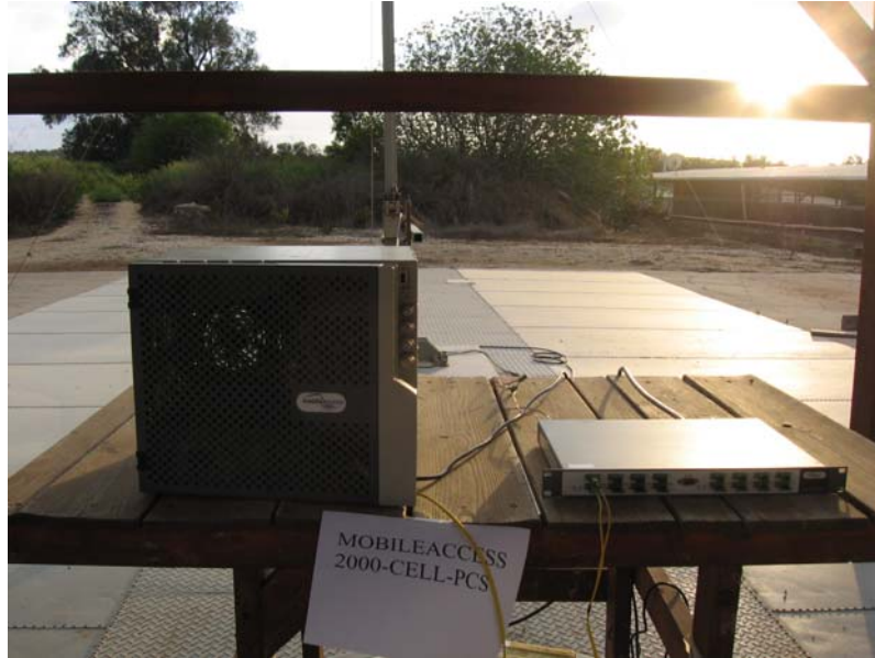
Figure 4. Radiated Emission Test Set-up
