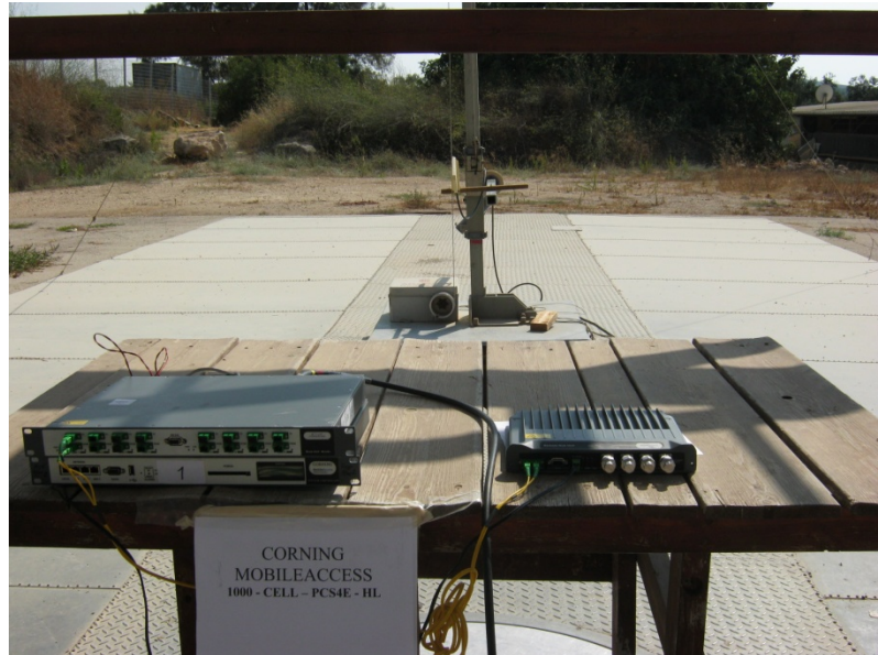
Figure 3. Conducted Emission From Antenna Ports Tests
