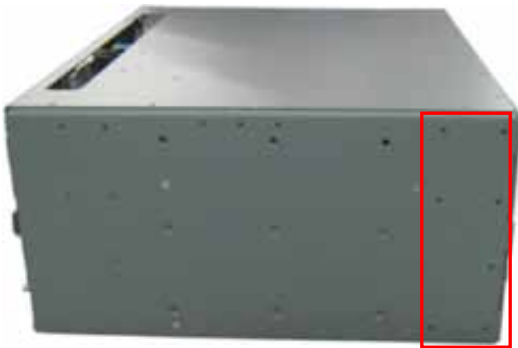
Figure 3-9. Holes for Securing Wall Mount Bracket
