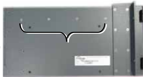
Figure 4-2. Side View of cabinet – remove screws
