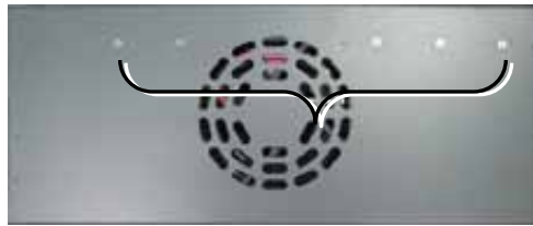
Figure 4-3. Rear View of cabinet – remove screws
