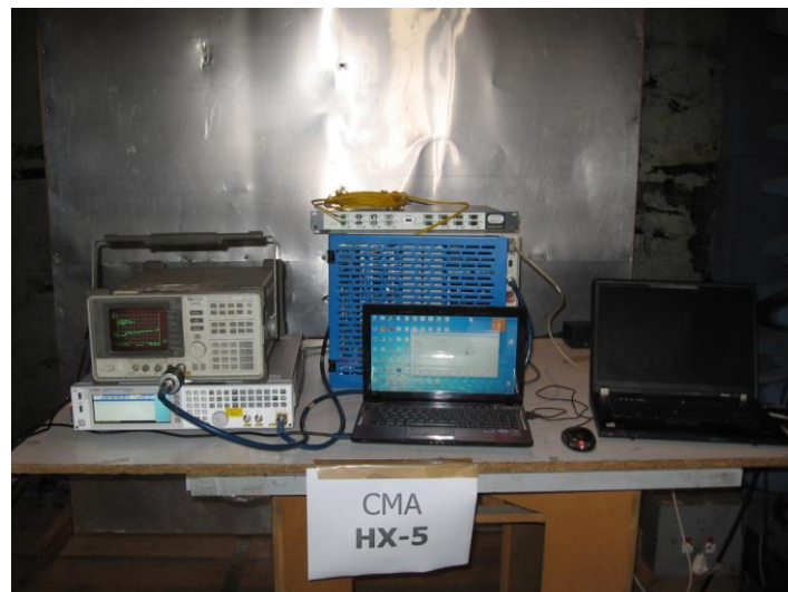
Figure 3. Conducted Emission From Antenna Ports Tests
