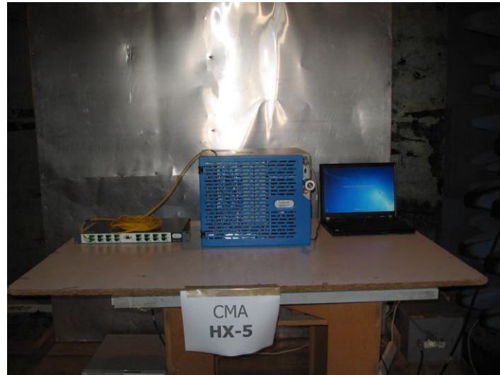
Figure 2. Conducted Emission From AC Mains Test
