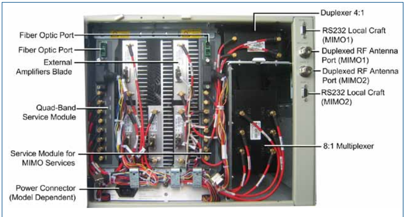
Example of HX Indoor MIMO Remote Unit Internal View (Front)
