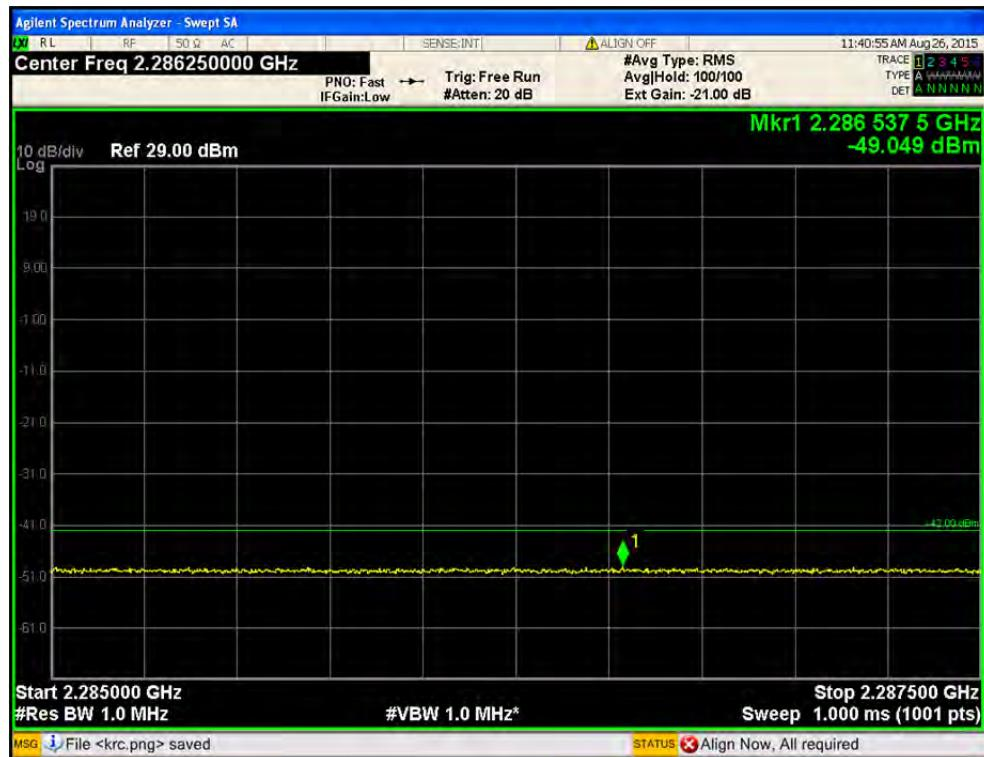
**• Port2 / LTE 5 MHz / 2 357.5 MHz / 64QAM / below 2 285.0 MHz**
