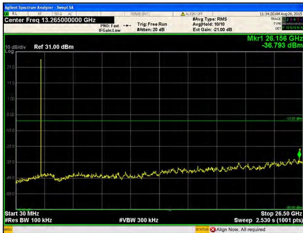
**• Port2 / LTE 5MHz / 2 357.5 MHz / 64QAM / 30 MHz ~ 26.5 GHz**
