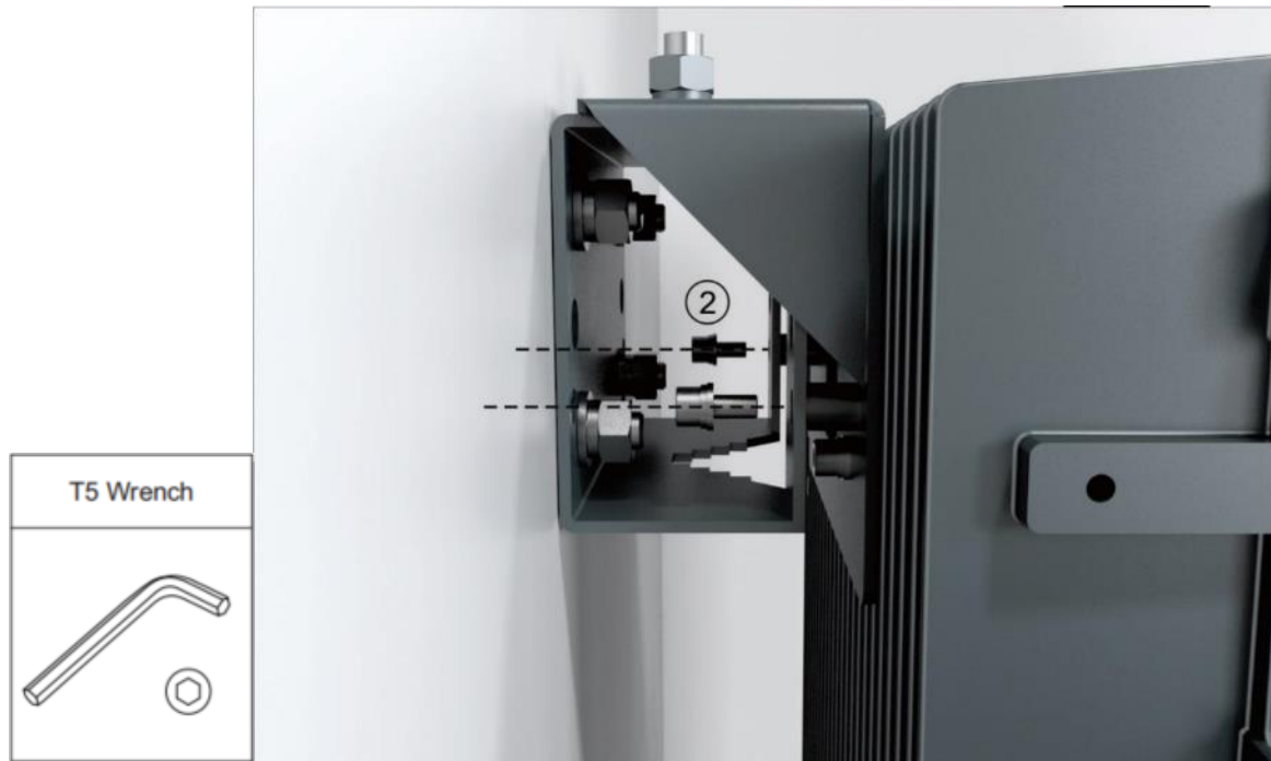
Figure 35. Fasten the Bracket I and II
