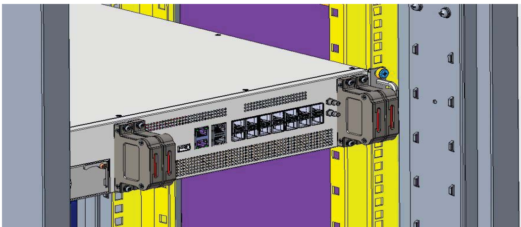
Figure 30. DCU RF Cable Plug Installation
