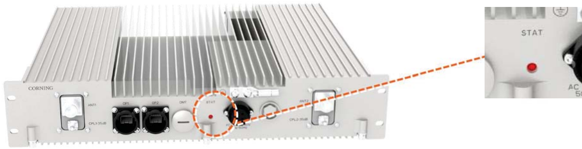
Figure 73. LED on DMRU
