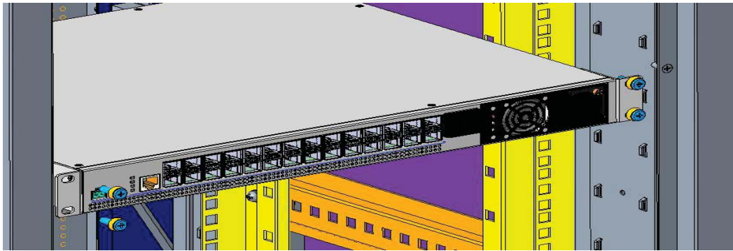
Figure 33. Rack Installation - Step 2
