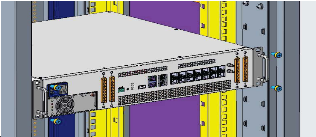
Figure 29. Installation Diagram of DCU in the Rack
