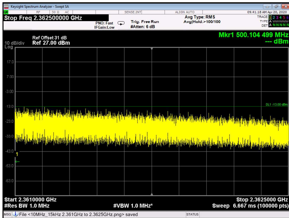
Figure 96: Spurious Emissions at Antenna Terminal 256QAM, 2355.0MHz, B.W. 10MHz, Sub Carrier 30kHz
