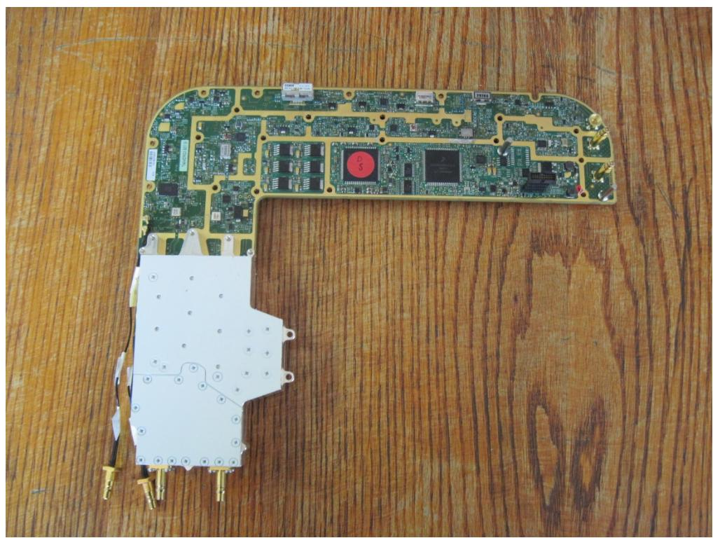
RF cavity filter with cover removed that is connected to end of PCB
