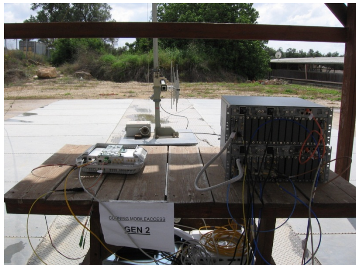
Figure 5. Radiated Emission Test
