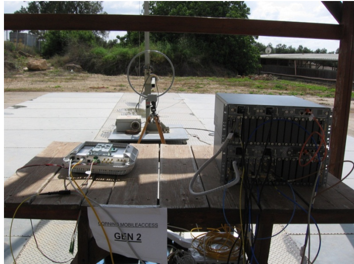
Figure 4. Radiated Emission Test
