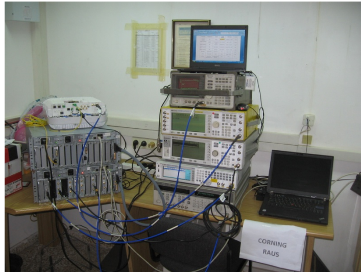
Figure 2. Conducted Emission From Antenna Port Tests
