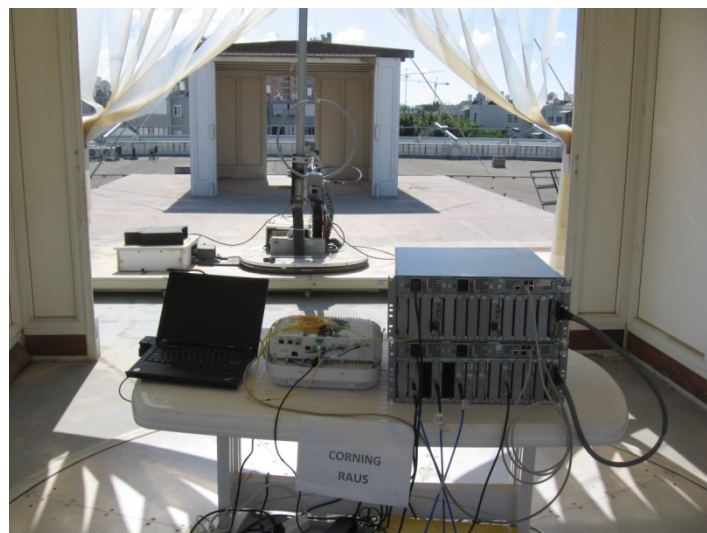
Figure 3. Radiated Emission Test
