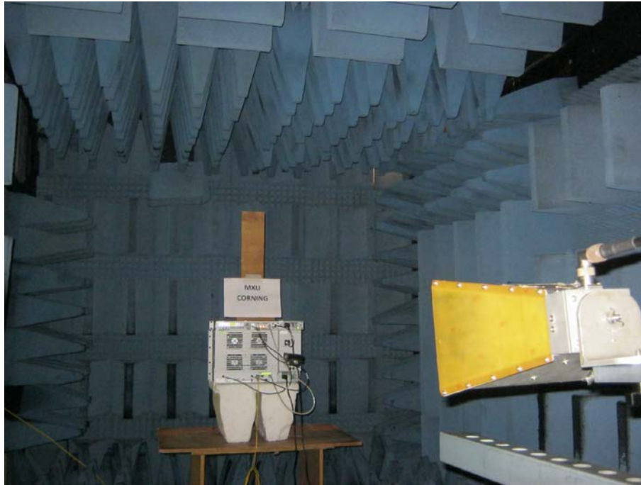
Figure 7. Radiated Emission Test – above 1GHz
