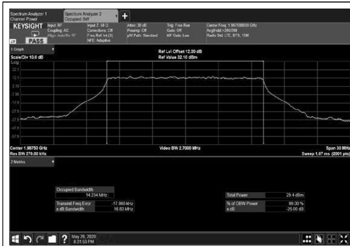
Figure 259: 64QAM 15MHz B.W.; 1987.5MHz, 15kHz Output
