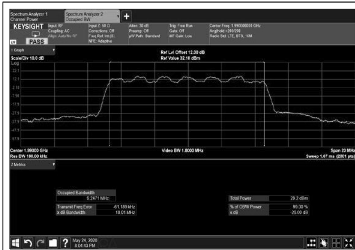
Figure 217: 16QAM 10MHz B.W.; 1990.0MHz, 15kHz Output
