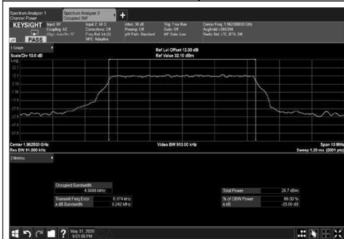
Figure 273: 256QAM 5MHz B.W.; 1962.5MHz, 15kHz Output
