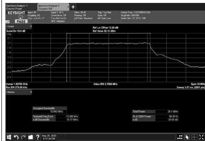
Figure 255: 64QAM 15MHz B.W.; 1937.5MHz, 60kHz Output
