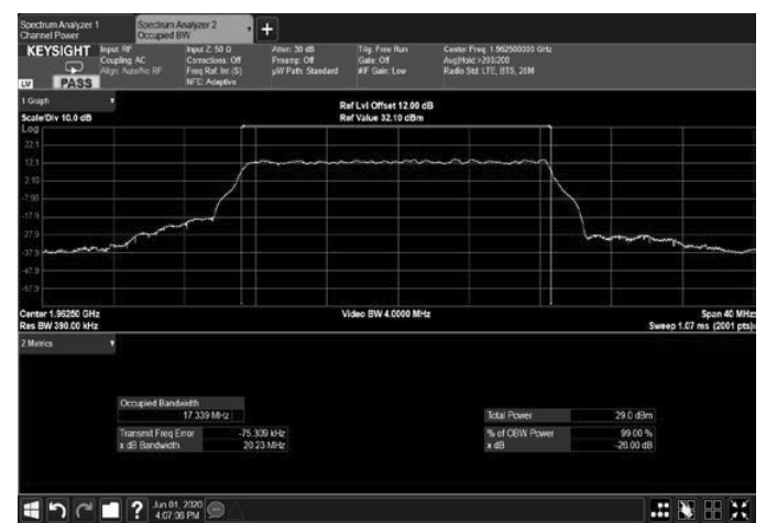
Figure 300: 256QAM 20MHz B.W.; 1962.5MHz, 60kHz Output
