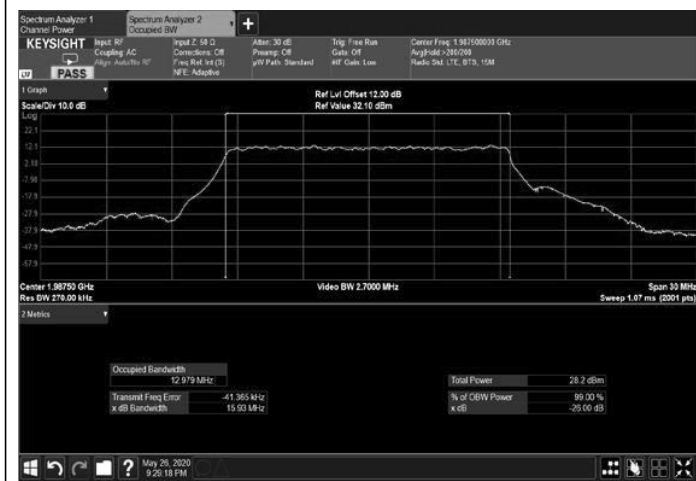
Figure 261: 64QAM 15MHz B.W.; 1987.5MHz, 60kHz Output
