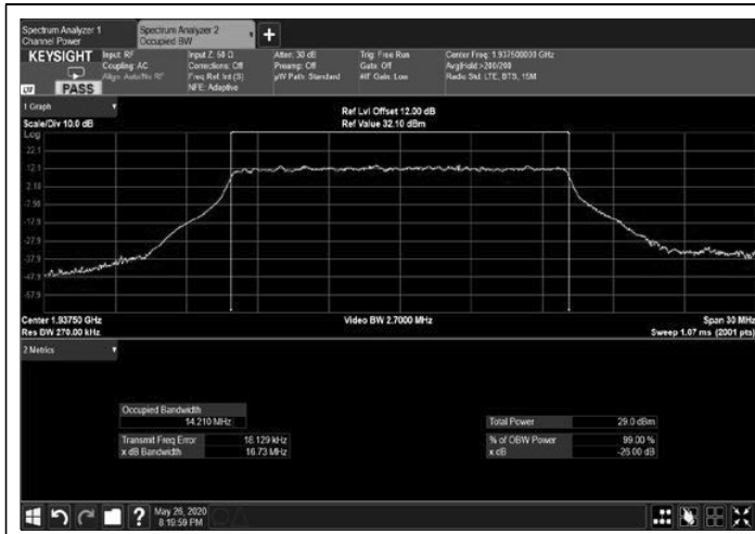
Figure 253: 64QAM 15MHz B.W.; 1937.5MHz, 15kHz Output
