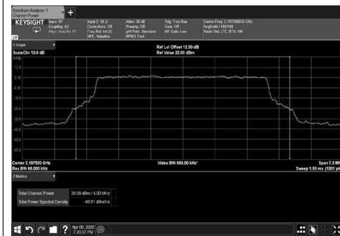
Figure 45: 64QAM 5MHz B.W.; 2197.5MHz, 30kHz
