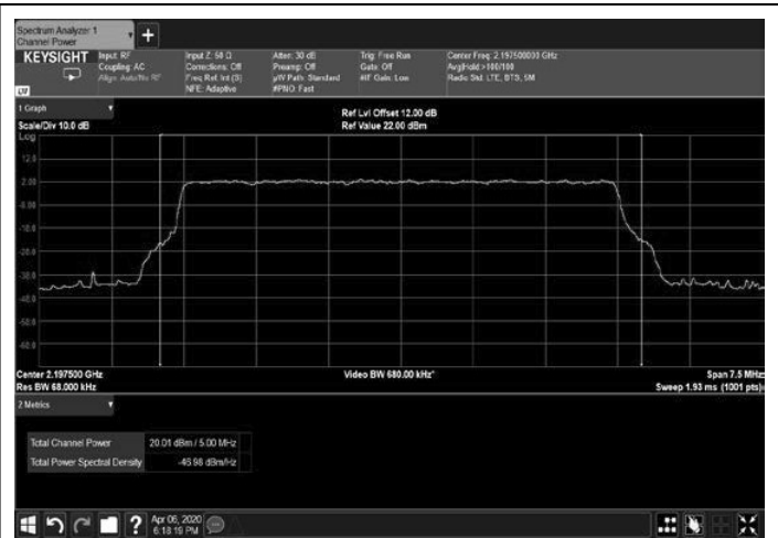
Figure 44: 64QAM 5MHz B.W.; 2197.5MHz, 15kHz
