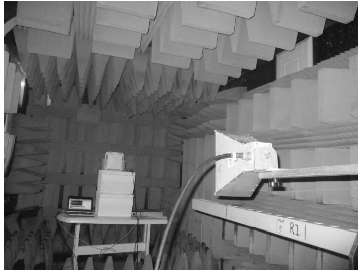
Figure 5. Radiated Emission Test 1-18GHz
