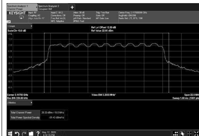
Figure 23: 16QAM 15MHz B.W.; 2117.5MHz, 30kHz
