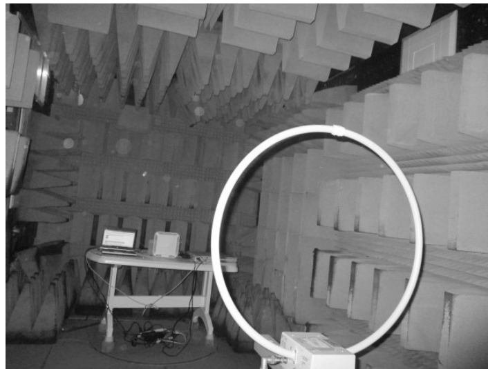
Figure 2. Radiated Emission Test 9kHz - 30MHz
