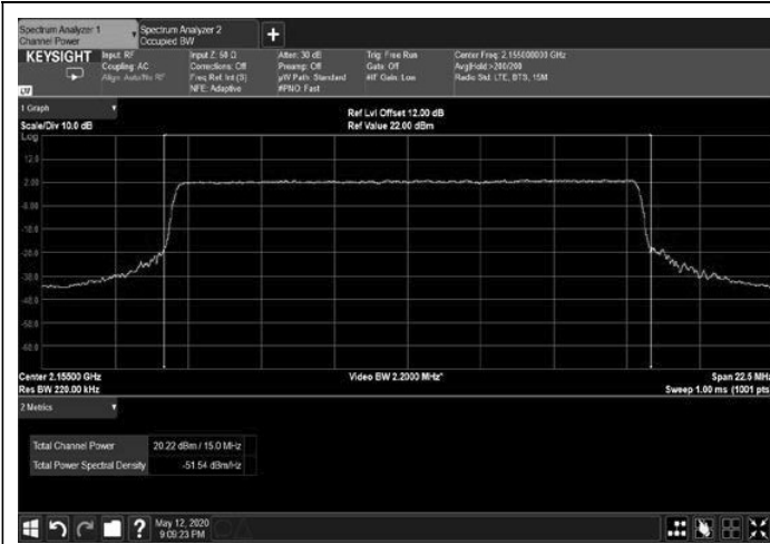
Figure 91: 256QAM 15MHz B.W.; 2155.0MHz, 15kHz
