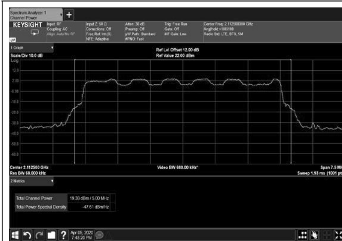
Figure 7: 16QAM 5MHz B.W.; 2112.5MHz, 15kHz
