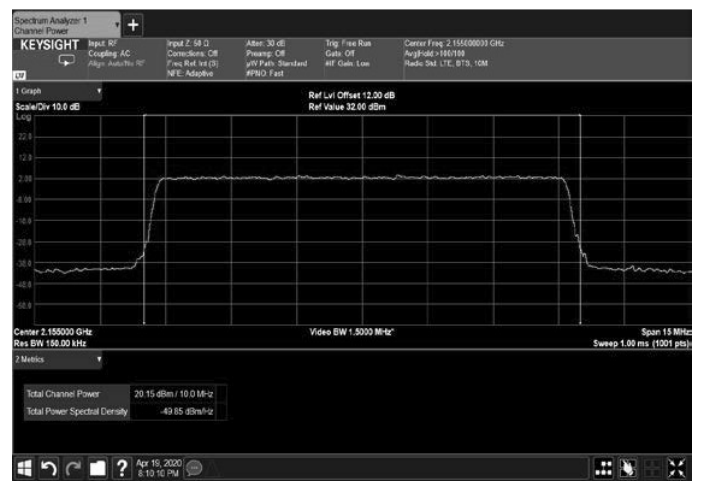
Figure 82: 256QAM 10MHz B.W.; 2155.0MHz, 15Hz
