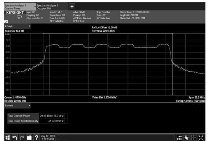
Figure 22: 16QAM 15MHz B.W.; 2117.5MHz, 15kHz
