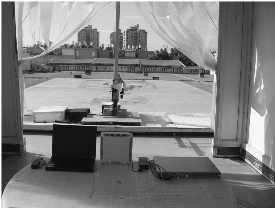
Figure 4. Radiated Emission Test 200 - 1000MHz
