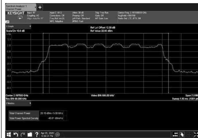
Figure 11: 16QAM 5MHz B.W.; 2197.5MHz, 15kHz
