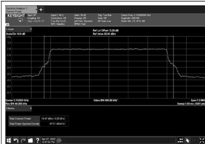
Figure 73: 256QAM 20MHz B.W.; 2112.5MHz, 15kHz
