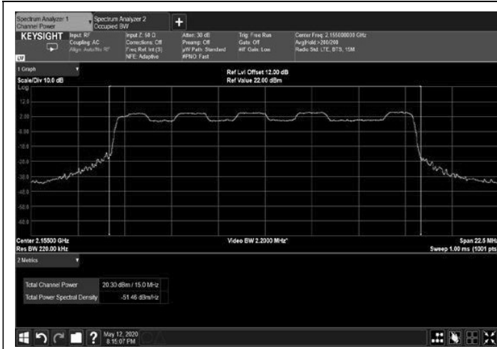
Figure 25: 16QAM 15MHz B.W.; 2155.0MHz, 15kHz
