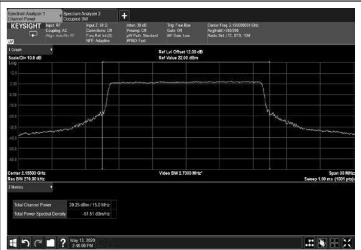
Figure 92: 256QAM 15MHz B.W.; 2155.0MHz, 30kHz
