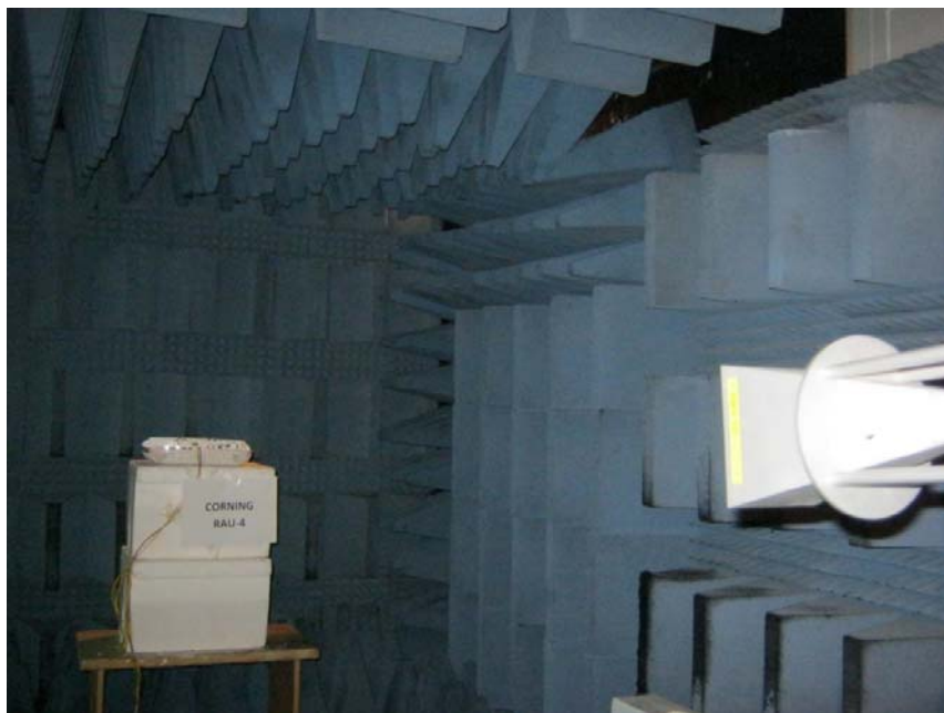
Figure 8. Radiated Emission Test
