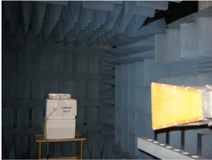
Figure 7. Radiated Emission Test
