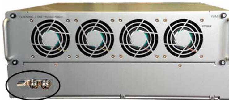
Figure 5-29. OIU Grounding Lug (Chassis Rear)
