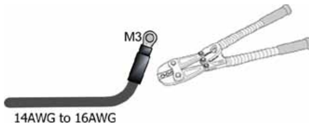
Figure 5-19. Crimping the Terminal Rings onto the DC Wire
