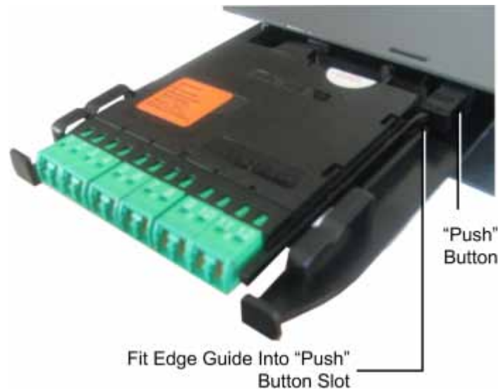
Figure 5-44. Inserting Edge Module (Chassis Front)
