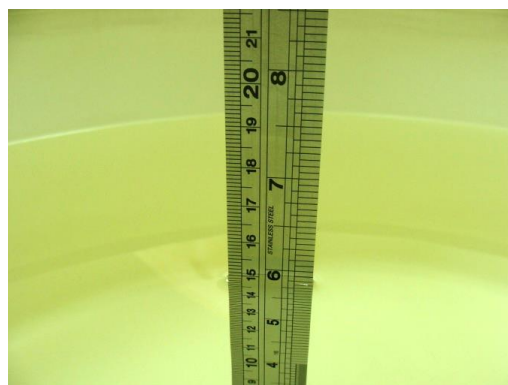
Fig 6.2 Photo of Liquid Height for Body SAR
