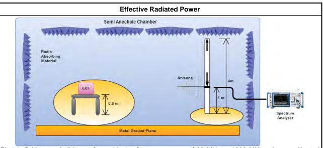
Electric field tests shall be performed in the frequency range of 30 MHz to 1000 MHz using a calibrated bi-log antenna and the frequency range of 1 GHz to 40 GHz using a calibrated horn antenna.
