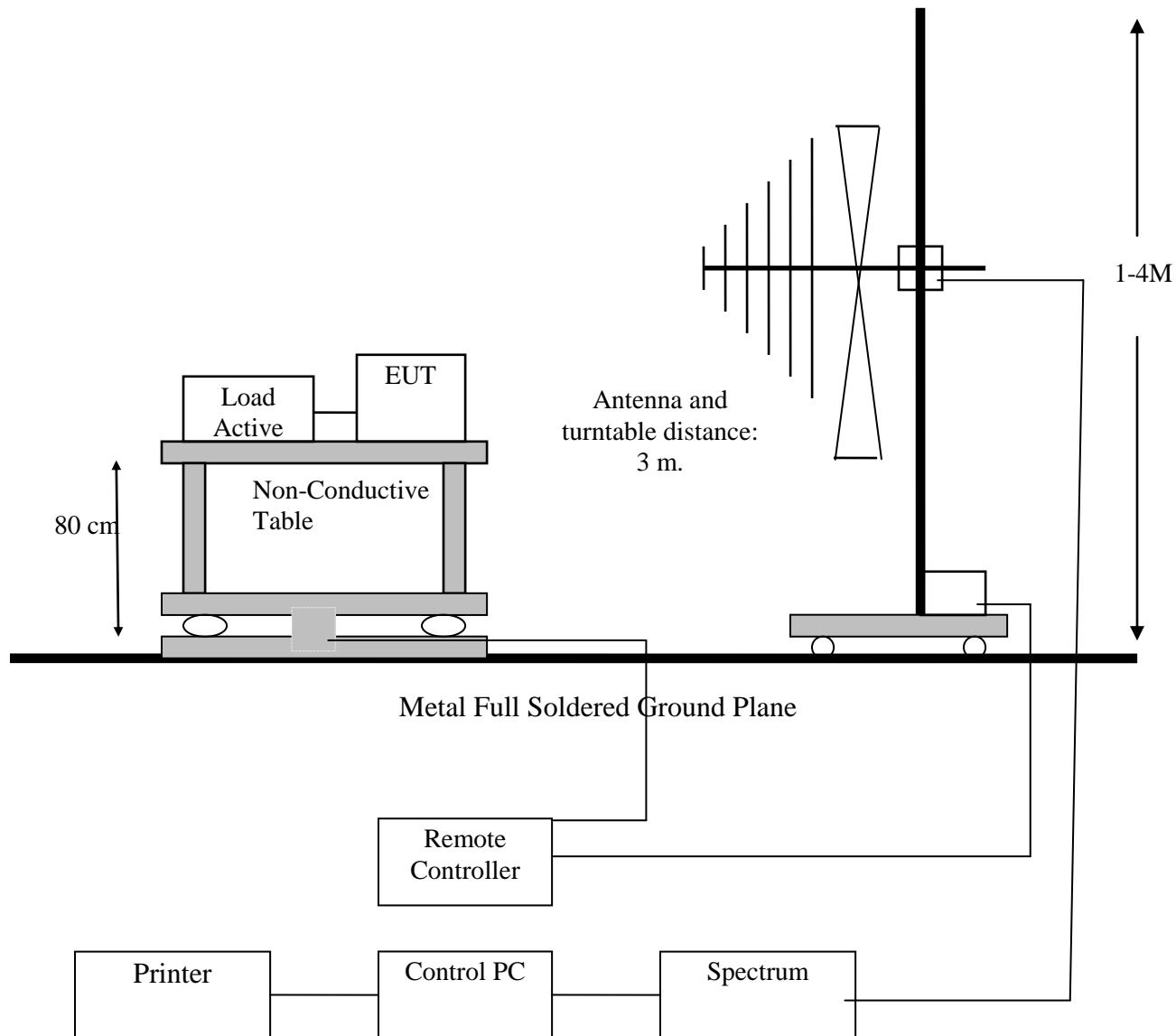
The test setup for emission measurement above 1 GHz
