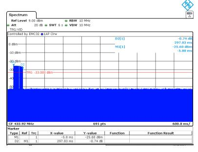
3. Regulation 15.231 (a2) A transmitter activated automatically shall cease transmission within
