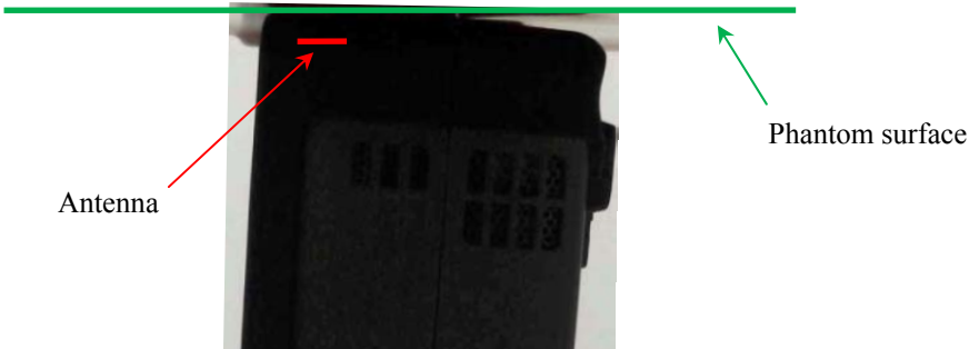
Closest condition of antenna to phantom surface distance. (In this test configuration, tilt slightly EUT.)
