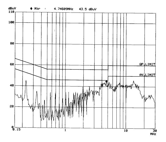
ADT CORP. SHIELDED ROOM A CISPR22 CLASS B EUT: LEGO Cam-001 Op Cond: EPP MODE Report No.: F88031961 Test Spec: LISN:N Comment: 120V AC / 60Hz Page: 11-2 Date: 22. Mar 99 11:24 Test By: ) aico Tenq Overview Scan Settings (3 Ranges) Start Stop Step IF BW Detector M-Time Atten Preamp 3.90625k 3.90625k 3M 150k 9k PK 10ms 10dBLN OFF 3M 10M 9k PK 0.05ms 10dBLN 0FF 10M 30M 3.90625k 9k PΚ 0.05ms 10dBLN **OFF** Stop Transducer No. Start Name 1 150k 30M C\_CA\_01A
