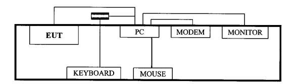
Both conducted and radiated testing were performed according to the procedures in ANSI C63.4:1992. Radiated testing was performed at an antenna to EUT distance of 10m on an open area test site. Please refer to the photos of test configuration in Item 5.
