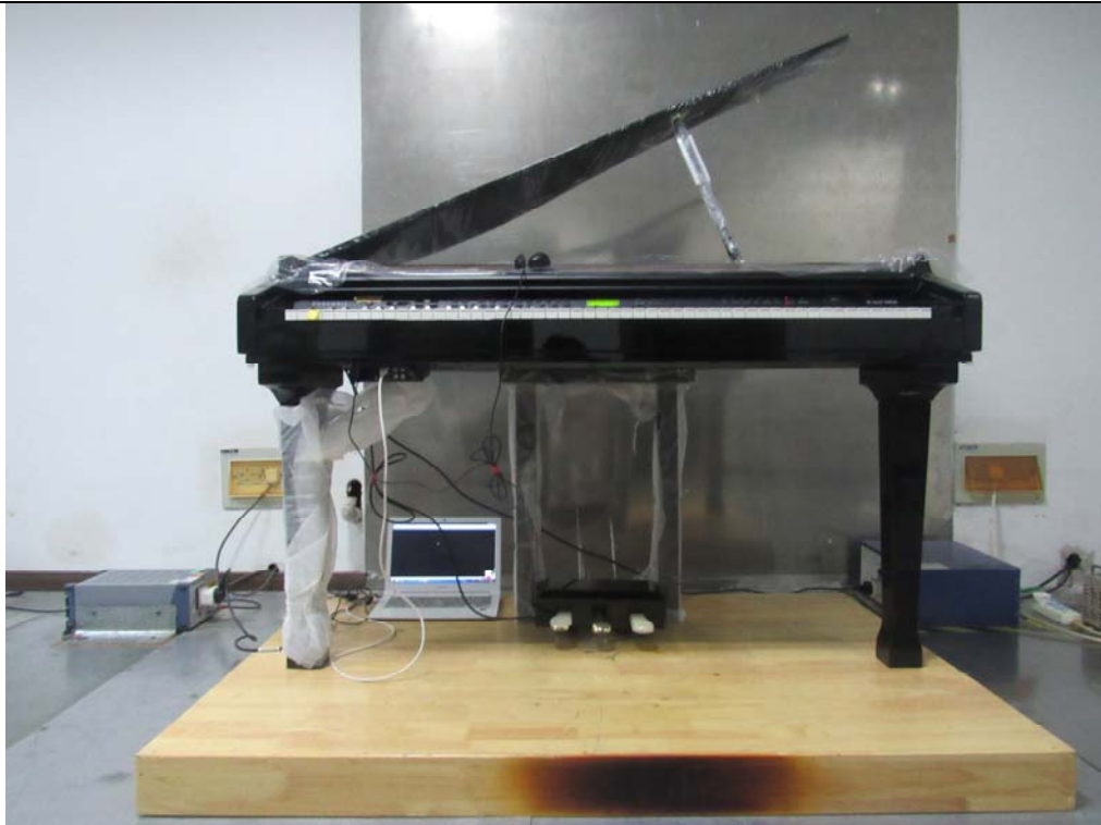
Conducted Emissions Setup Front View
