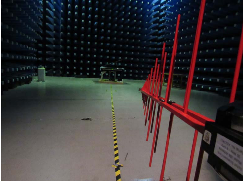
Radiated Emissions Setup Below 1GHz Front View
