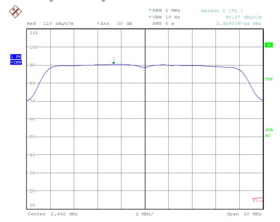
Note: The correction factor is already included in the spectrum analyzer as a transducer factor so that the marker shows directly the field strength level.
