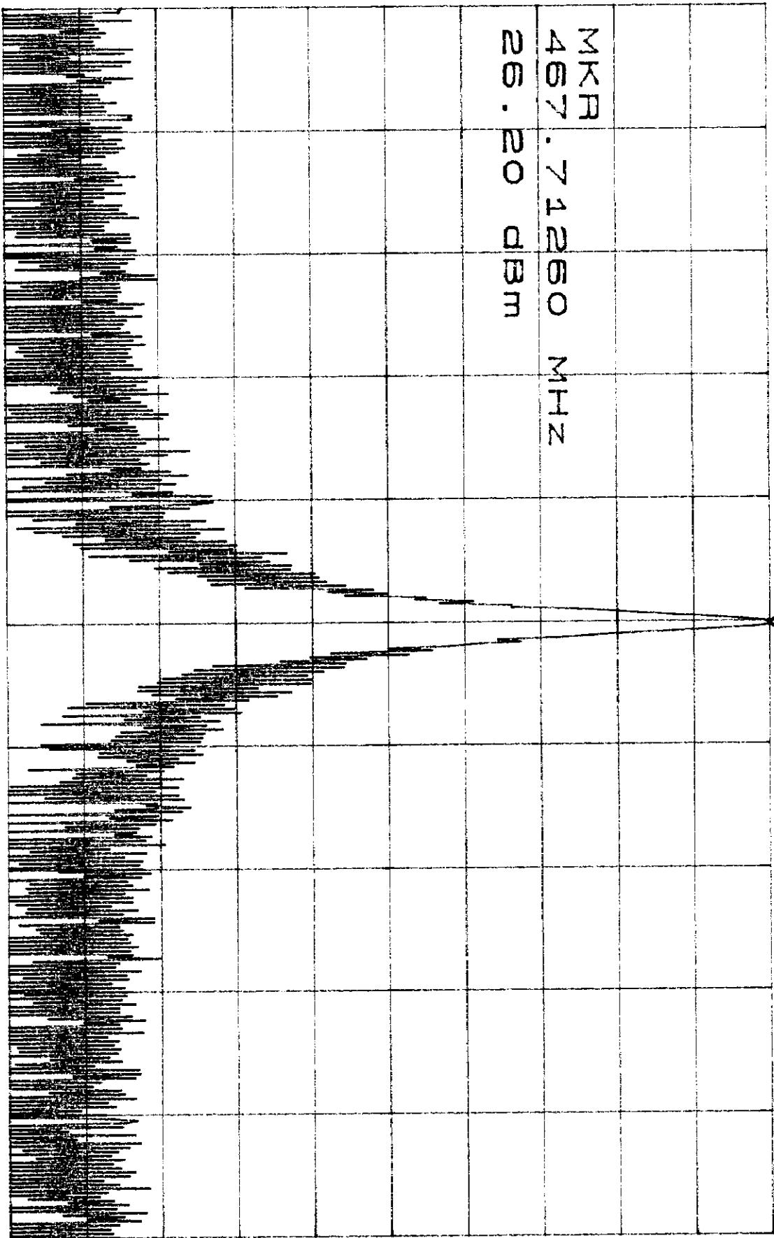
CENTER 467.71250MHz SPAN 62.50KHz
