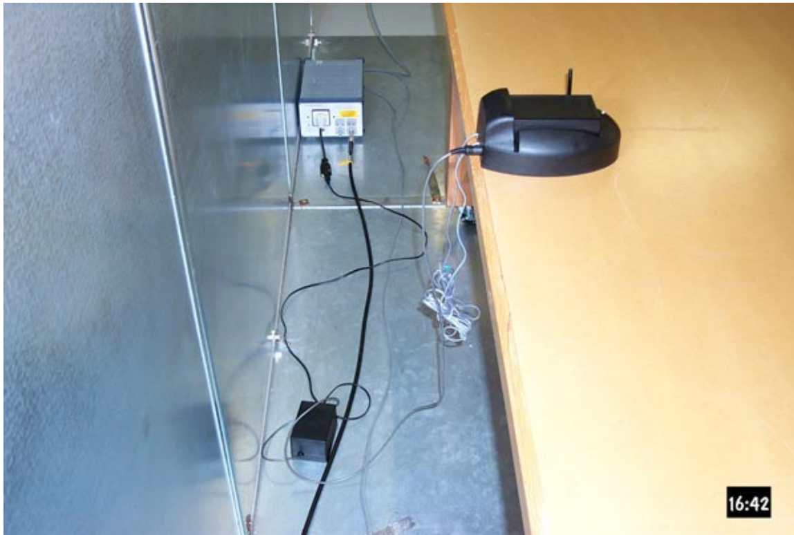
Figure 1 Conducted Emissions test setup
