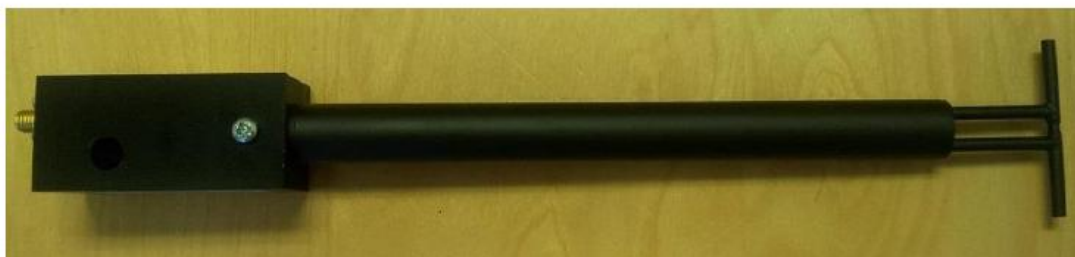
Figure 1 – MVG COMOSAR Validation Dipole
