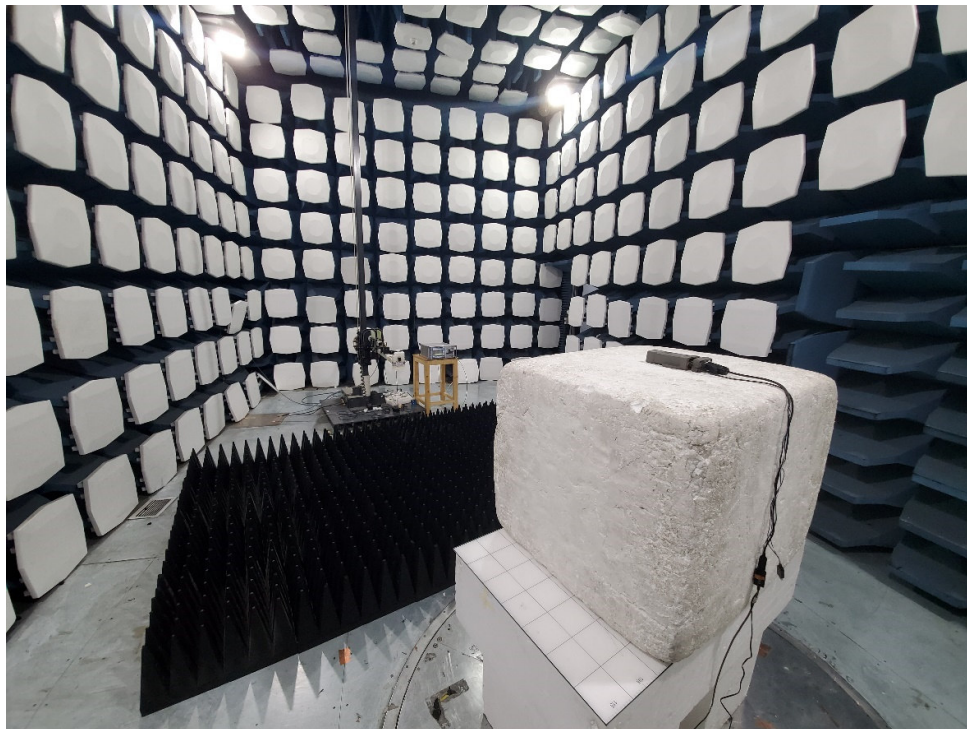
Picture 1: Radiated Spurious Emissions Test setup
