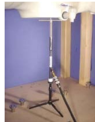
900MHz System Check Setup
