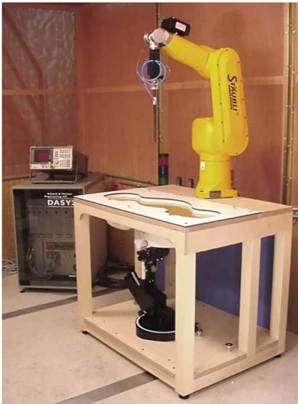
DASY3 SAR Measurement System with SAM Phantom
