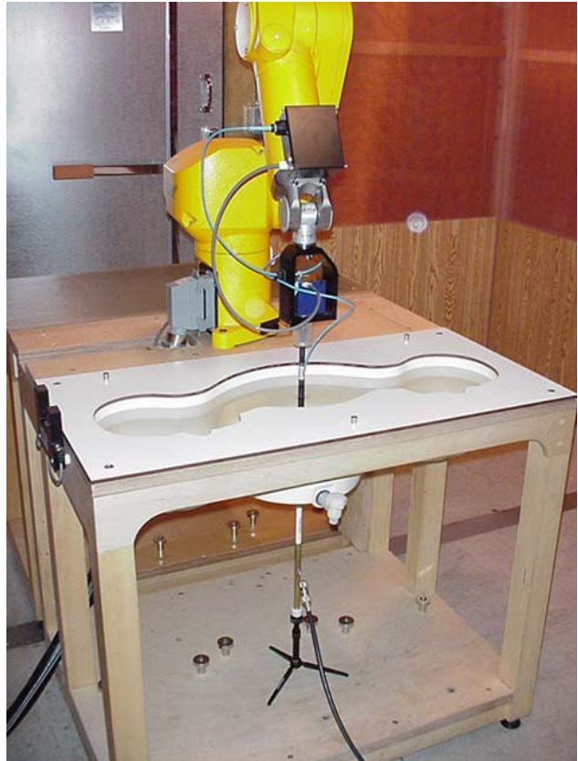
DASY4 Measurement System with SAM Phantom
