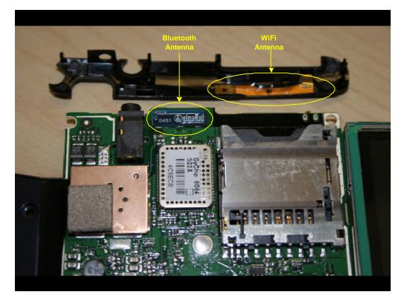
4) Even thought the RF portions are a secondary module boards, bottom views of the module boards are still required. It is not necessary to destroy the sample to take these, but instead take from an uninstalled part. Please provide.
